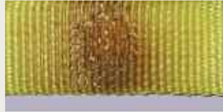
Melting or charring of the tie down, or weld splatter on the tie down
